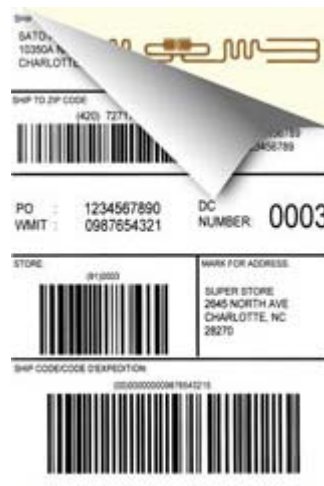
Figure 13: Example of Smart Label that Could Be Affixed to a Shipping Container Complying with the JAIF B-16 Global Transport Label Standard for the Automotive Industry
